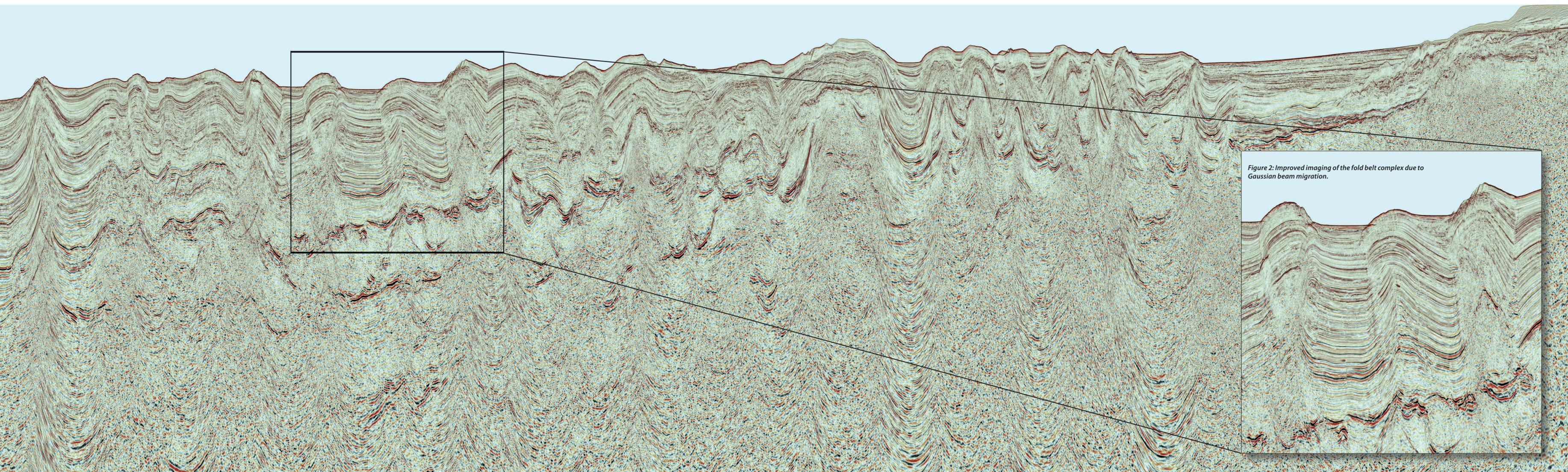
Figure 2: Improved imaging of the fold belt complex due to Gaussian beam migration.
