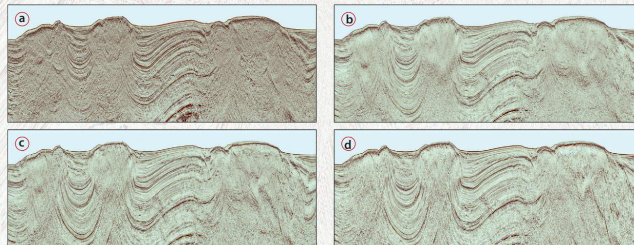
Figure 6: Image of pre-salt section. (a) Original KPSDM; (b) New KPSDM; (c) New GBM; (d) New RTM Mid Frequency.
